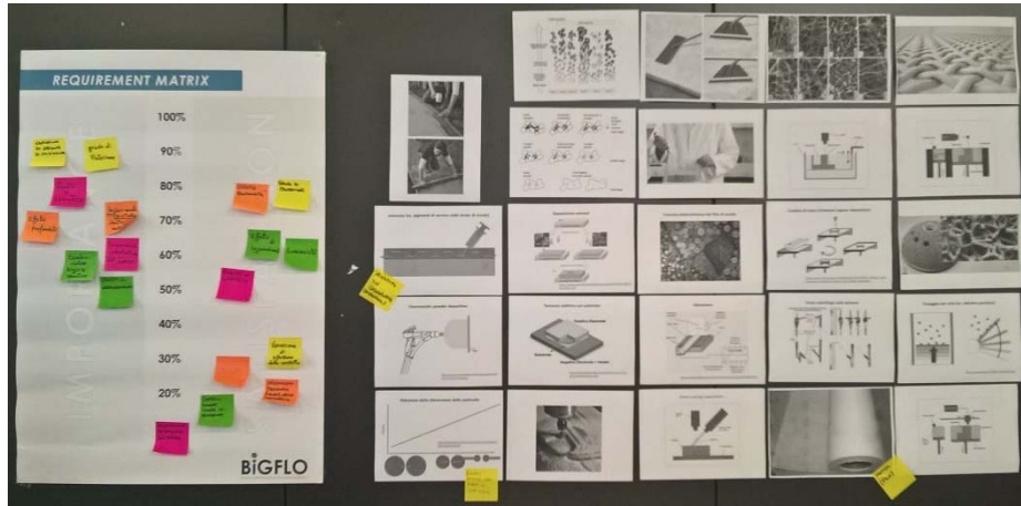
Fig. 1. An example of the tools (requirement matrix on the left and visual triggers on the right) used to analyze the problem and explore the space of the solutions.
